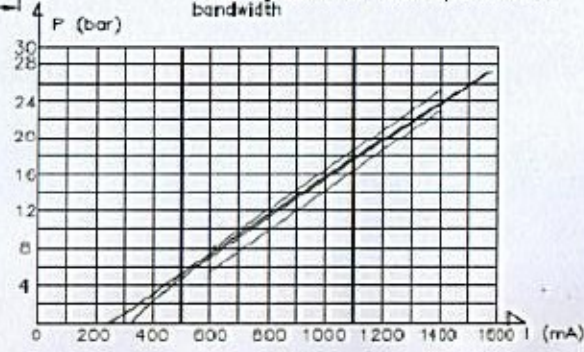
PRESS. VS. CURRENT CHARACTERISTIC 12 VDC coil / 5.4 ohm - T oil 50°C boundary limits of the response curve bandwidth
